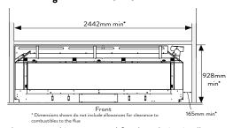
Note: These are minimum cavity framing dimensions and may not achieve a centred fireplace design in all specifications. Please adjust overall cavity size if required.
