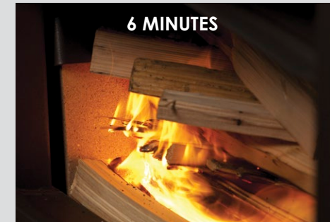
Igniter shuts down and blower continues to push air acting as bellows to fan the fire
